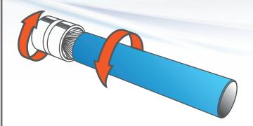
Chamfer end of tube
