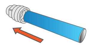
Push tube into seat of fitting
