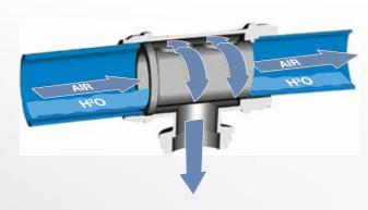
The Zero Condensate Tee provides the advantage of automatically reducing the size of the ring main to a smaller drop leg diameter, making the need for extra fittings obsolete. Its internal geometric shape means that it can be used vertically or horizontally, and the internal barrel may be rotated by 360° for off shoot lines. Additionally, in many cases, the Zero Condensate Tee may replace a coupler when placed appropriately.
